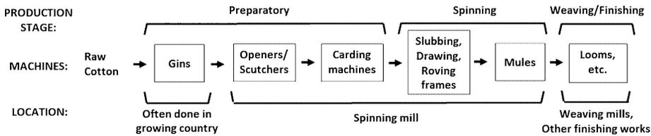
FIGURE 1.—The cotton textile production process.
